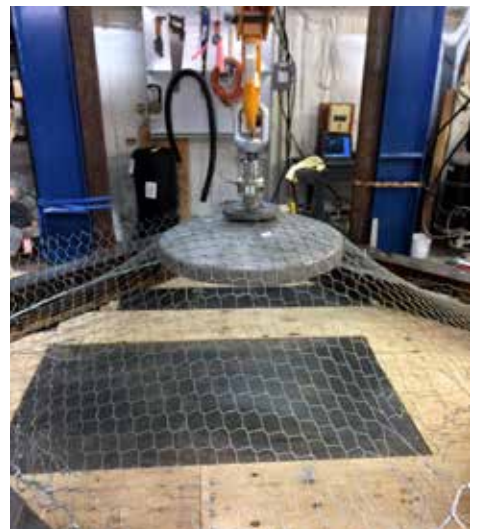
TRI rockfall mesh "Punch" puncture resistance test with 1 meter diameter probe
