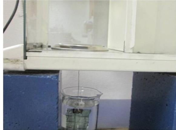
Figure 9. Specific gravity measurements require a highly accurate scale.
