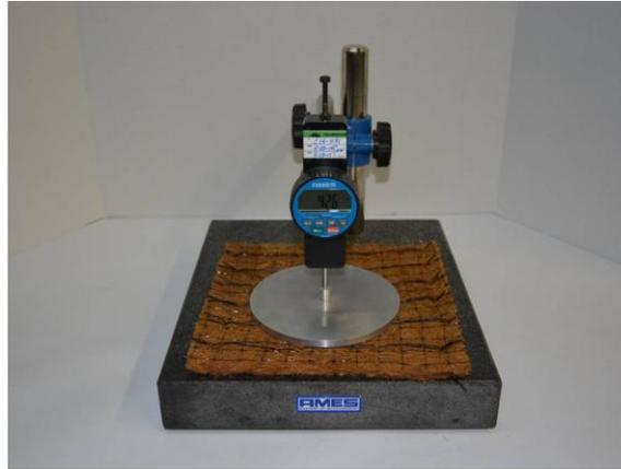
Figure 5. Thickness measuring apparatus.
