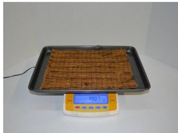
Figure 4. Weigh specimens (after oven drying if ECB)
