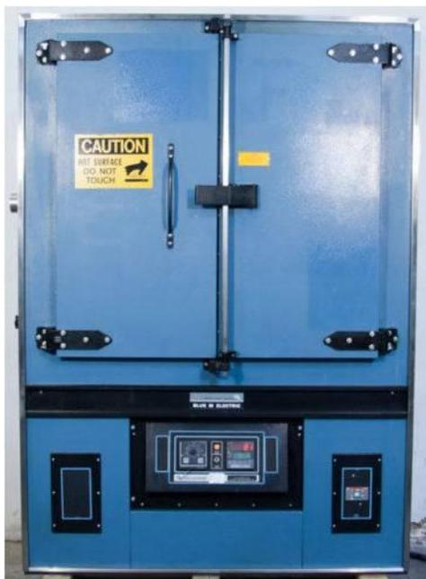
Figure 3. Temporary RECP specimens are oven dried.
