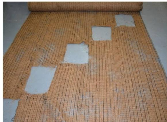
Figure 1. Specimens or coupons are cut from the sample across the roll width
