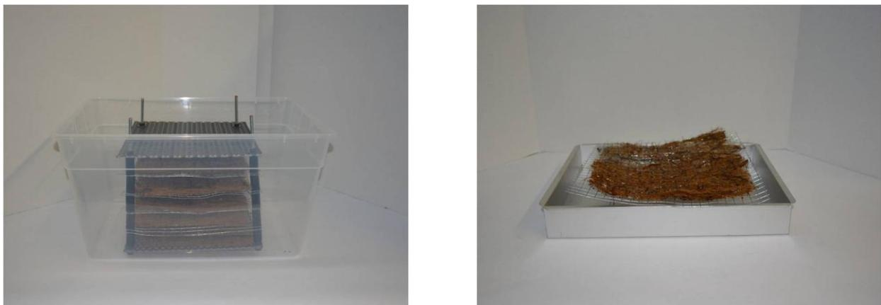
Figure 8. Conditioned samples are weighed, soaked, drained, and weighed
