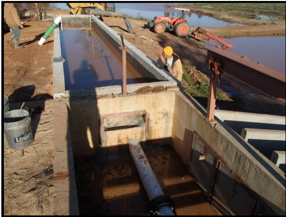
Figure 6. View of Test Pool during Fill Test
