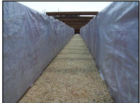
Figure 8. RECP Secured to Soil in Flume and Ready for Testing
