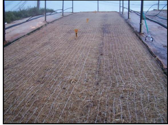
Figure 4. RECP Being Tested On Slope
