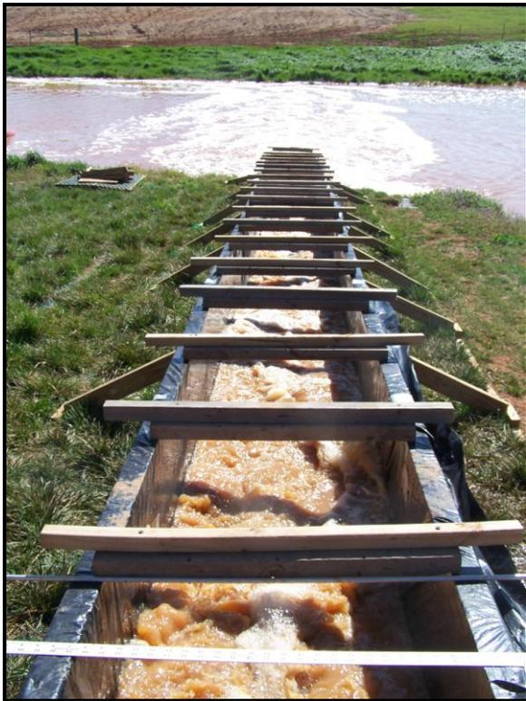
Figure 7. 10% Flume for Higher Shear Levels
