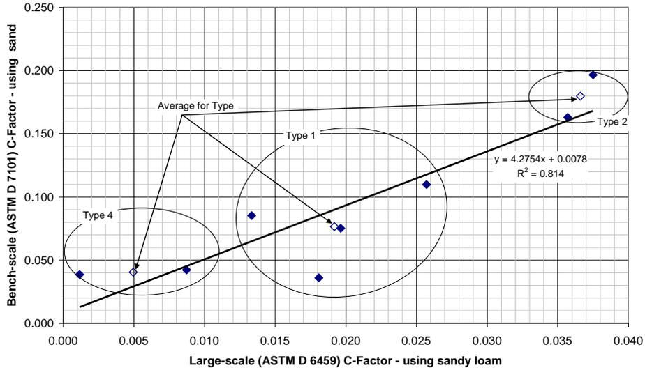
Figure 10. Bench-scale vs. Large-scale Slope Results
