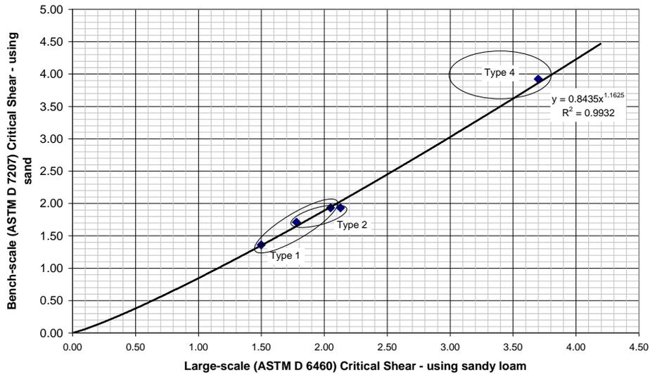
Figure 11. Bench-scale vs. Large-scale Channel Shear Results
