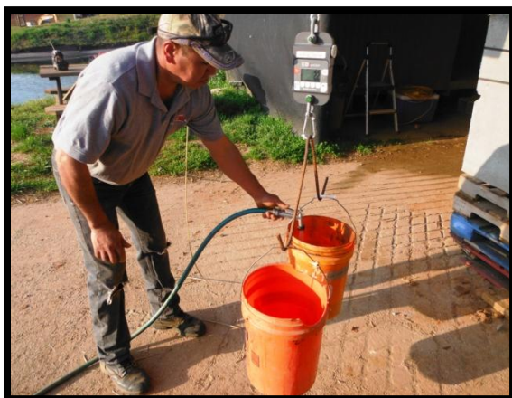
Figure 5 – Load Application with Load Cell Visible
