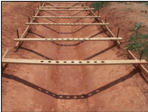
Figure 1. Flume Setup (typical control)
