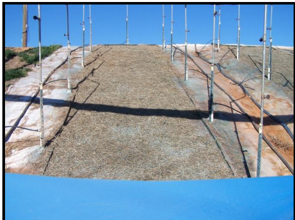
Figure 9. Typical "Tacked Straw" Test Slope – Before Test and Nearing Test Completion
