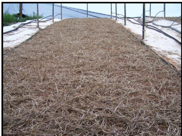
Figure 10. Typical "Crimped Straw" Test Slope – Before Test and Nearing Test Completion
