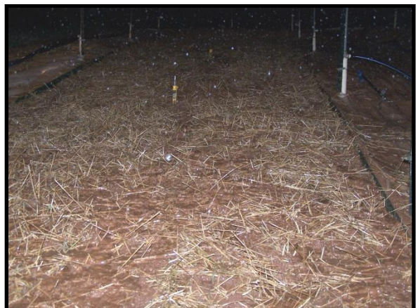
Figure 10. Typical "Crimped Straw" Test Slope – Before Test and Nearing Test Completion
