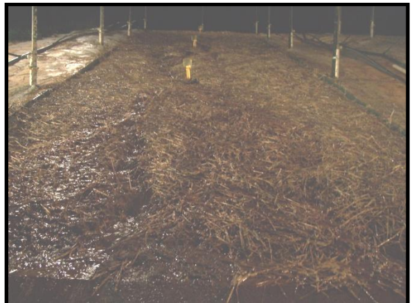
Figure 9. Typical "Tacked Straw" Test Slope – Before Test and Nearing Test Completion
