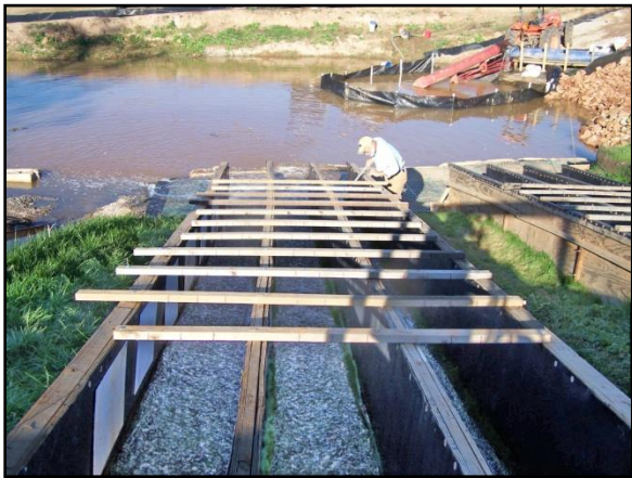
Figure 2. 6+ Week Vegetated Shear in 20% Flumes; Recirculation Pump in Background
