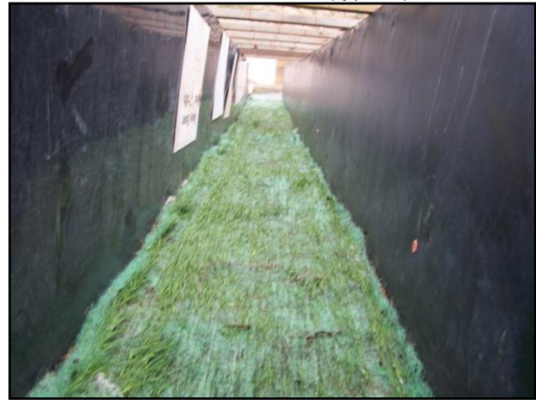
Figure 11. 6+ Week Vegetated Channel after Test (typical)
