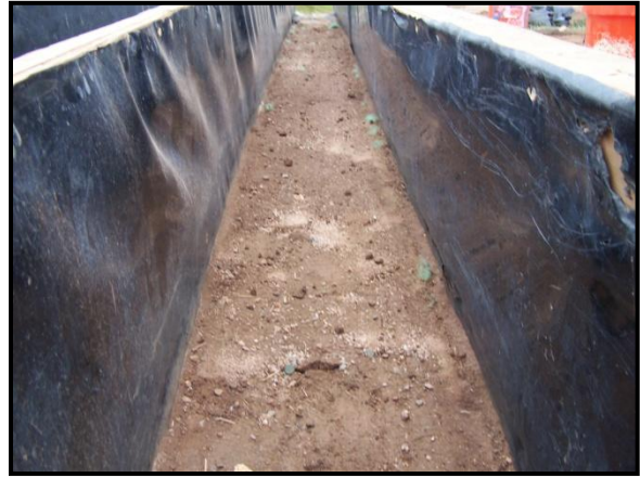
Figure 10. Unvegetated Channel after Test with Product Removed (typical)
