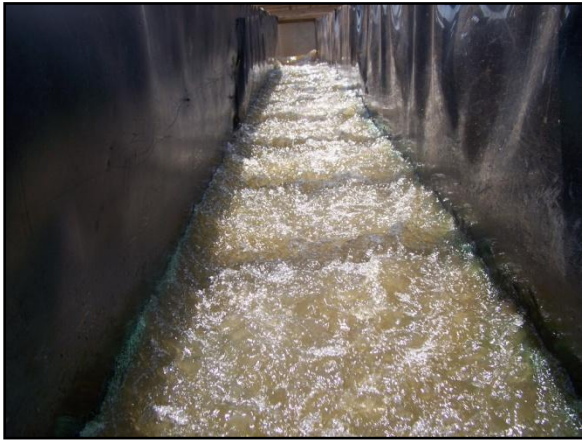
Figure 7. Typical Flow in Unvegetated Channel
