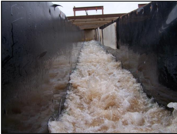
Figure 8. Typical Flow in 6+ Week Vegetated Channel
