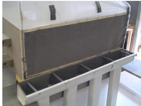
Figure 2. Close-up of Silt Fence Testing Setup
