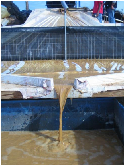
Figure 4. Full-scale Sediment Control Testing "System" with a High Flow Silt Fence System
