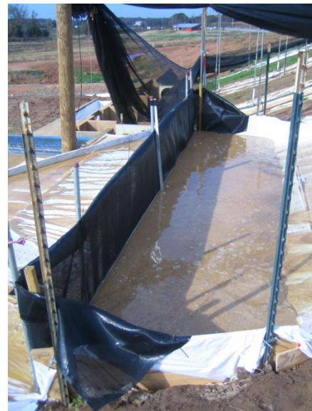
Figure 5. Full-scale Sediment Control Testing "System" Showing Modest Impoundment with a High Flow Silt Fence System
