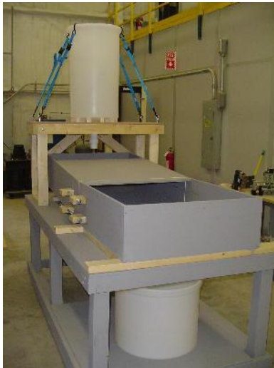
Figure 1. Bench-scale Sediment Control Testing Apparatus (with Horizontal “Box” Extension for Testing Inlet Filter Systems)
