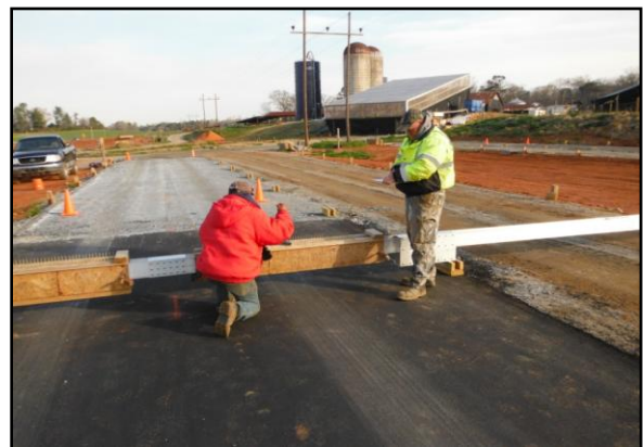
Figure 6. Centerline Deflection and Rut Measurement
