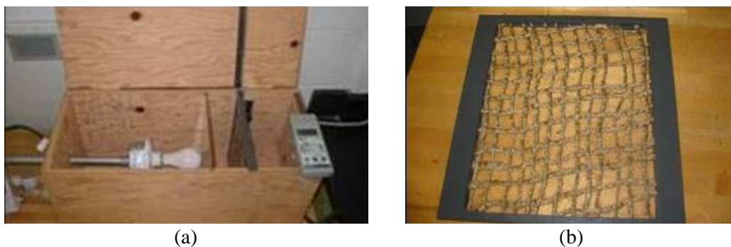
Figure 2. Light penetration (a) apparatus and (b) specimen in the testing frame
