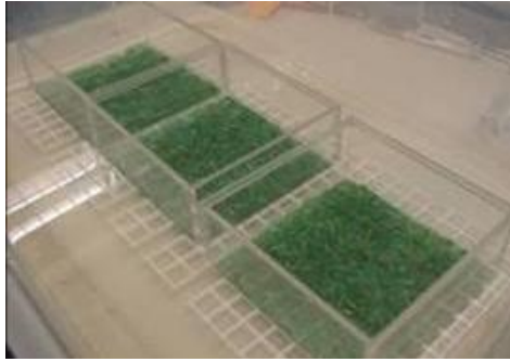
Figure 10. Water uptake (a) reservoir with three specimen containers
